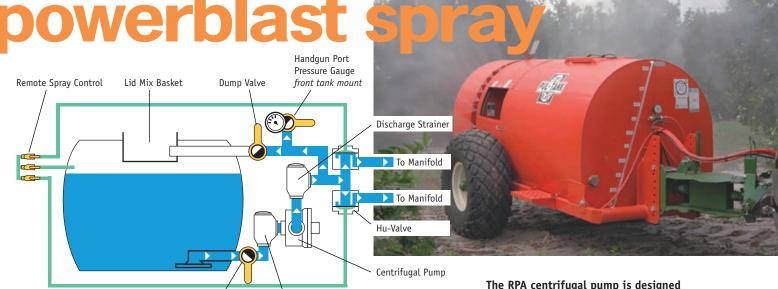
The plumbing of the Powerblast was designed for ease of operation and maintenance: during and between applications.
