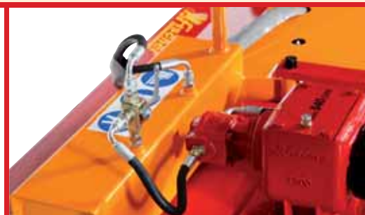
Self supply pump and tank
